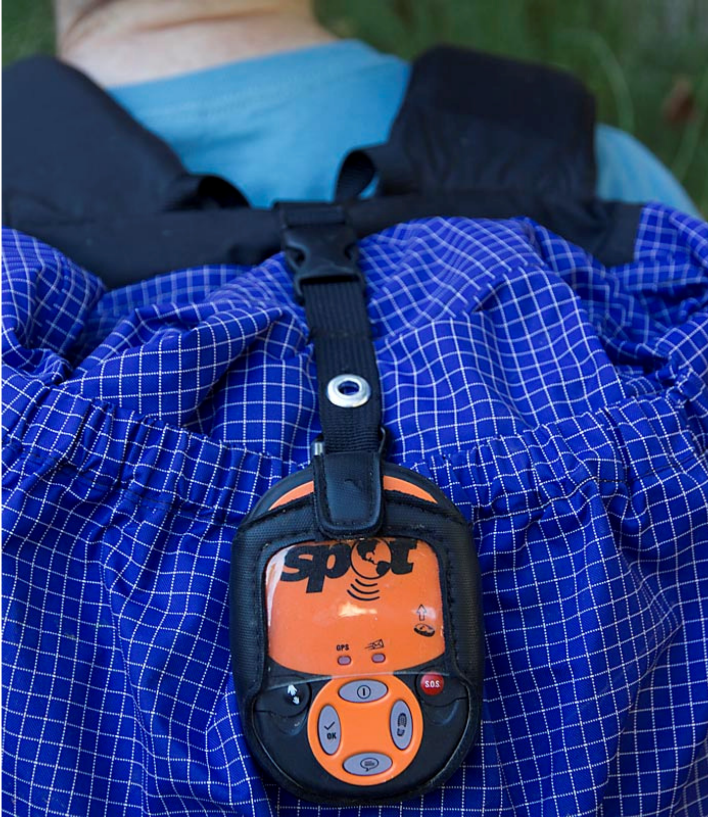
Lazy person's vertical mounting of the SPOT2 used when field testing in a southern Utah
