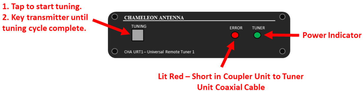
Figure 10. Coupler Unit Operation.
