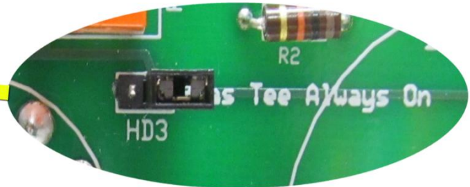
Bias Tee Shown NOT jumpered Factory Default
