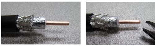
Most RG-213 type cables with a solid polyethylene dielectric will cut properly using the tool, but the end part of the dielectric that needs to be removed may be strongly adhered to the center conductor(s). Some will twist off, others may need to be slit to break it loose from the center conductor. Take care to avoid damaging the center conductor(s). The photos below show this method to remove the dielectric without damaging the center conductors.
