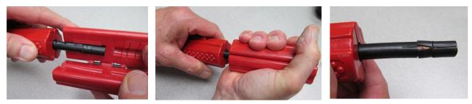
4. Remove the two pieces of the coax jacket on the end to expose the center insulator. Some of the braid may still be present. Use the DXE-170M Precision Braid Trimmers to cut the braid even with the second cut as shown.
