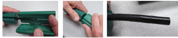
3. Place the prepped coax cable into the other side of the pre tool that has the single blade. While gripping and firmly squeezing both the cable gripper and the tool pull the cutter off of the coaxial cable. This action puts a single length-wise slit in the coaxial cable jacket.
