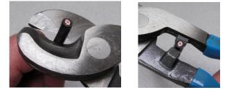
2. Place the coaxial cable in the tool on the end that has the three blades as shown. Use the Cable Gripper to help hold the coaxial cable. While holding the tools parallel to each other, squeeze the gripper to hold the coax and squeeze the cutting to make the initial cut in the coax. Rotate the coax cutter a few turns around the coax while squeezing to make the three cuts complete.
