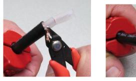
5. Remove the end piece of the dielectric (see the "Notes about Coaxial Cables" on page 7) and peel off the last part of the cut jacket to expose the braid. Gently flare it out slightly and install the crimp style connector under the braid. Ensure the center conductor is straight so it will go into the center conductor of the connector.
