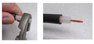
This example shows cutting the dielectric to remove it from the center conductor strands.
