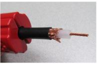
6. Slip the connector onto the coaxial cable under the braid, then slip the coax connector ferrule into place. Crimp the ferrule and you're ready to solder the center pin to complete the installation.
