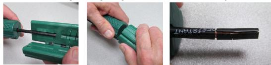
4. Remove the two pieces of the coax jacket on the end to expose the center insulator. Some of the braid may still be present. Use the DXE-170M Precision Braid Trimmers to cut the braid even with the second cut as shown.
