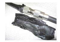
Looking at the removed weatherproofing, you can see the 3M Temflex<sup>TM</sup> 2155 Rubber Splicing Tape fully conformed to your connector assembly and fully protected the connectors when properly applied as described in this guide.
