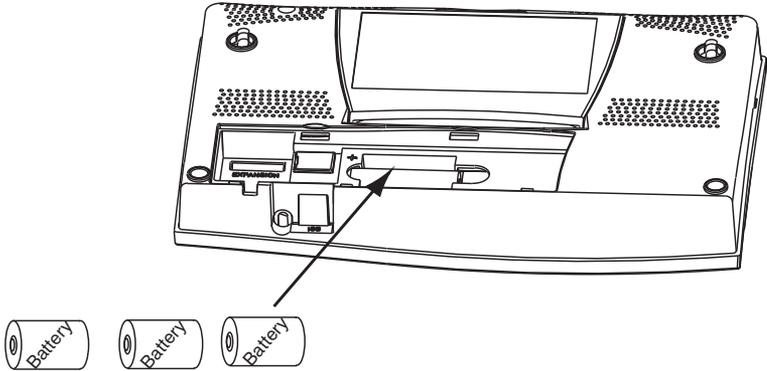
2. Insert three C batteries into the battery channel, negative (or flat) terminal first.
