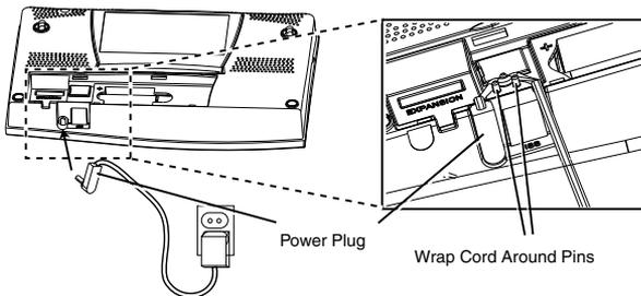
3. Insert the power adapter plug into the console power jack, then plug the other end of the adapter into an appropriate power outlet.
