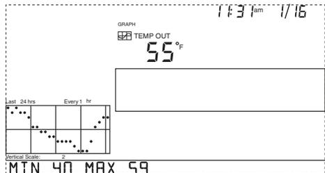
The screen displays the new dot's value. The time display shows what hour of the last 24 is being viewed.
