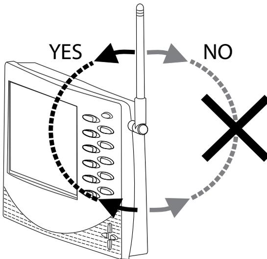
Wireless consoles have an antenna that rotates 180° **forward**. It is important that you do not over rotate the antenna by forcing it backward beyond the up or down positions.
