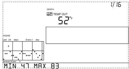
By pressing the - key again, the graph shifts to show the highs of the last 24 months. As before, use the < and > keys to move between months. Press HI/LOW to shift between the highs and lows.
