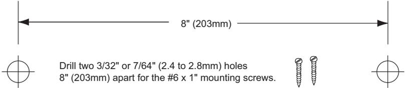
**This is a representation for the mounting hole positions. This template is not true to size.**
