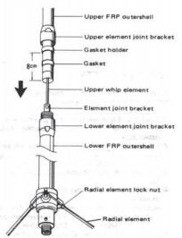
Fasten upper element and element joint bracket firmly.
