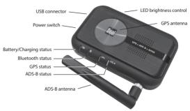
Please refer to the diagram above to locate the controls and indicators on the XGPS190.
