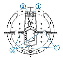
**4** Press the cables into any of the guide grooves ③ on the bottom of the case, and secure them using a cable hold-down plate ④.
