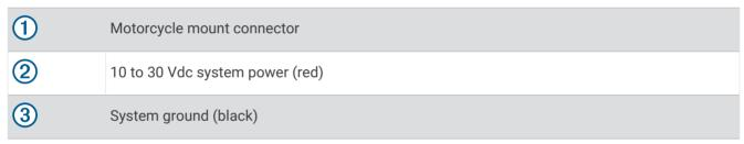
**NOTE:** Additional parts are included with the device to provide more installation and wiring options. Contact an experienced installer for more information about using these parts with your motorcycle.
