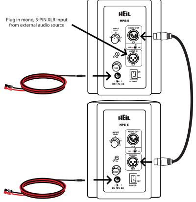
Note: The HPS-5 speaker is not meant to be used with a microphone plugged directly into the speaker.
