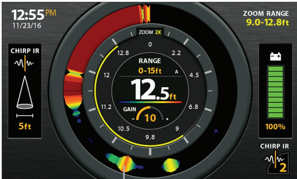
The size of the sonar returns correspond with the intensity of the sonar returns from the transducer beam(s).
