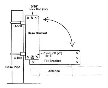
**Base Support:** Your base support pipe (not included with the ATB-75 kit) should be made from thick-wall steel or aluminum tubing and extend at least 3 to 4 feet below ground. For multi-band verticals, we recommend seating the pipe in a 10inch diameter posthole filled with ready-mix concrete to ensure stability. Note that antenna base supports should always be located well clear of power lines or neighboring property to avoid exposure to life-threatening injury or liability.
