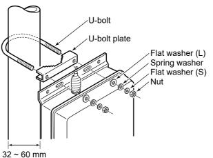
⚠ **WARNING!** Mount the AH-730 securely with the supplied nuts and bolts. Otherwise, vibrations and shocks could loosen the antenna tuner, making it fall, causing personal injury.
