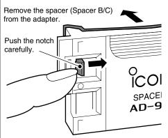
Push the notch carefully with your finger to remove the spacer (Spacer B/C) from the adapter (Spacer A).
