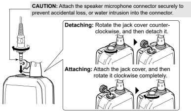
**NOTE: KEEP** the jack cover attached when the speaker microphone is not used. If the cover is not attached, water will get into the transceiver. Moreover, the terminals (pins) will become rusty, or the transceiver will function abnormally if the connector gets wet.
