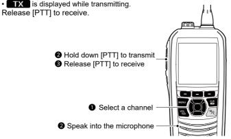
**TIP:** To maximize the readability of your transmitted signal, pause for a second after pushing [PTT] and hold the microphone 5 to 10 cm (2 to 4 inches) from your mouth, and then speak at your normal voice level.
