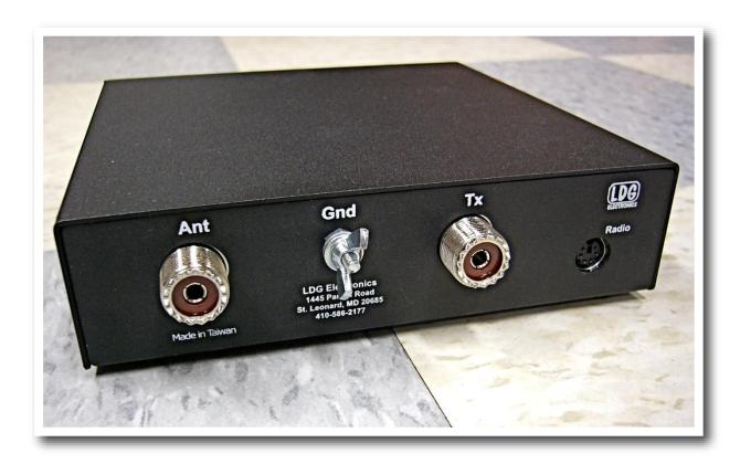
**GND connector (wing nut):** Connect to antenna system ground.
