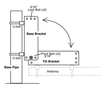
**Base Support:** Your base support pipe (not included with the MFJ-1903 kit) should be made from thick-wall steel or aluminum tubing and extend at least 3 to 4 feet below ground. For multi-band verticals, we recommend seating the pipe in a 10-inch diameter posthole filled with ready-mix concrete to ensure stability. Note that antenna base supports should always be located well clear of power lines or neighboring property to avoid exposure to life-threatening injury or liability.
