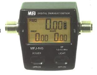
4. Forward power is displayed on the top of the screen while Reflected power is displayed on the bottom left of the screen and the SWR is displayed on the bottom right of the screen
