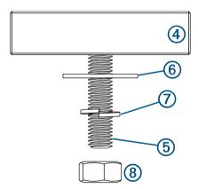
10 Using a torque wrench, tighten the nuts to 13.7 to 18.6 N-m (10 to 14 lbf-ft.).
