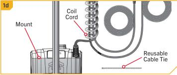
**NOTICE:** Minn Kota recommends routing the Accessory Cables through the Coil Cord. Bypassing the Coil Cord when routing Accessory Cables is not recommended.
