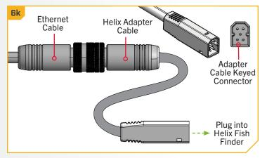
**NOTICE:** If unsure of what features the trolling motor may be installed with that require connection to an output device, please review the "Identifying Trolling Motor Features and Their Associated Cables" section of this manual.
