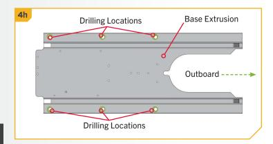
NOTICE: The mounting surface for the Ulterra QUEST must be flat. Rubber Washers can be used to shim the Base Extrusion flat before hardware is tightened.
