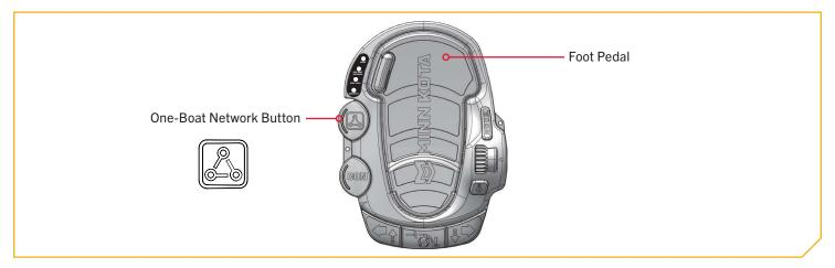
The One-Boat Network \Lambda button on the Foot Pedal can be customized to control the following functions:
