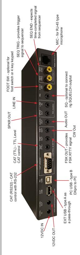
**Fixed-level RX audio cable**: This will take the place of the supplied stereo audio cable (steps 3 above) and will usually connect from a transceiver's accessory jack to LINE IN on the rear panel of the DXpro.
