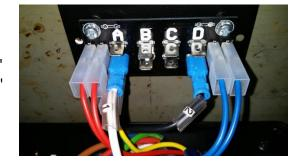
Connect cable "3" to one of the spade lugs labelled "A" Connect cable "4" to one of the spade lugs labelled "D"
