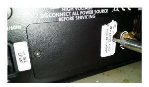
With a TORX (TX10) screwdriver, unscrew the left hand screw near the AC input connector.
