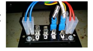
Connect cable "3" to one of the spade lugs labelled "B" Connect cable "4" to one of the spade lugs labelled "D"
