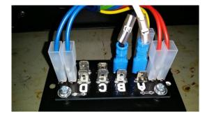
Connect cable "3" to one of the spade lugs labelled "B" Connect cable "4" to one of the spade lugs labelled "C"
