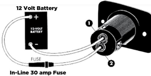
Mounting the receptacle requires a  $1\frac{1}{8}$ " hole to be drilled. Select a location where the boat's structure will not be weakened. Also, mount on a vertical surface to lessen the amount of water that can enter the receptacle.
