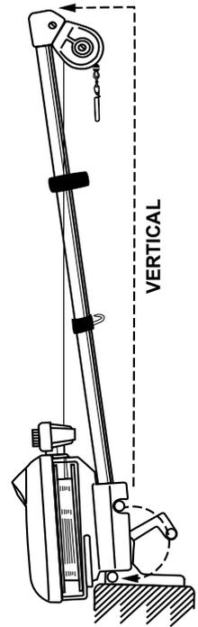
**Red lock lever must be tucked under base to lock the downrigger upright.**
