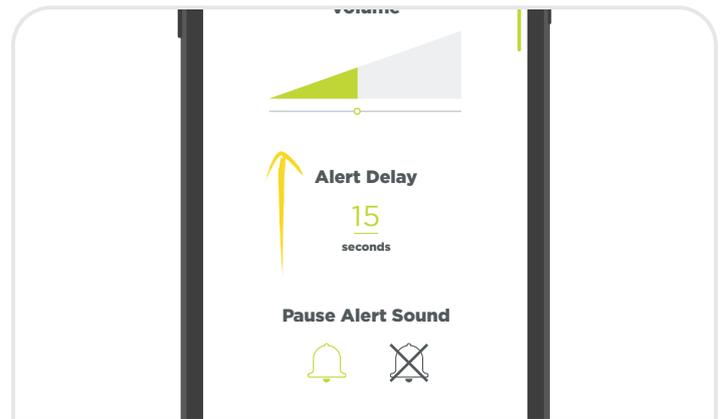
4. Adjust the Alert Delay to 15 seconds. This means if the connection between the Tag and the mobile device is broken for longer than 15 seconds the alarm will sound.
