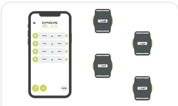
11. Ensure all OLAS transmitters are switched on and transmitting by checking the ID numbers on the home screen.
