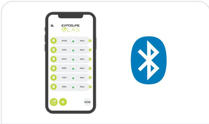
1. Ensure a maximum of 6 OLAS transmitters are being tracked. More than 6 OLAS transmitters within range will cause false alarms. If required, the addition of the OLAS Core or Guardian allows tracking of up to 15 OLAS transmitters. Disconnect any other Bluetooth devices from your mobile device. Remove any phone cases for testing purposes.
