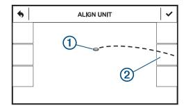
**10** Select the area at the edge of the screen ② where the clay enters the field of view.
