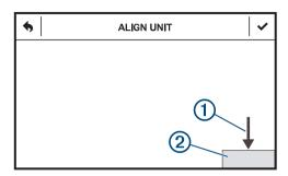
**NOTE:** The arrow and trap house could appear in different positions depending on your shooting station. You should verify the top of the alignment window is aligned with the top edge of the trap house.
