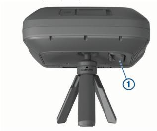
2 Release the tripod adjustment button to set the position.
