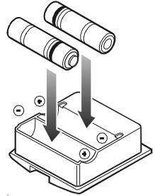
The **FBA-23** does not provide connections for charging, since Alkaline cells cannot be re-charged. Therefore, the **NC-72/PA-48**, **E-DC-5B**, or **E-DC-6** may safely be connected to the **EXT DC** jack when the **FBA-23** is installed.
